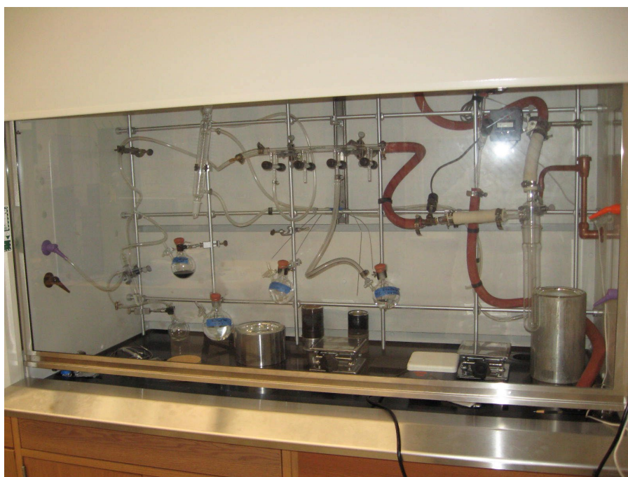
Figure 1: Appropriately used fume hood. Note the elevation of most of the equipment and the fact that only relevant equipment is present. Additionally, the sash is most of the way down.
