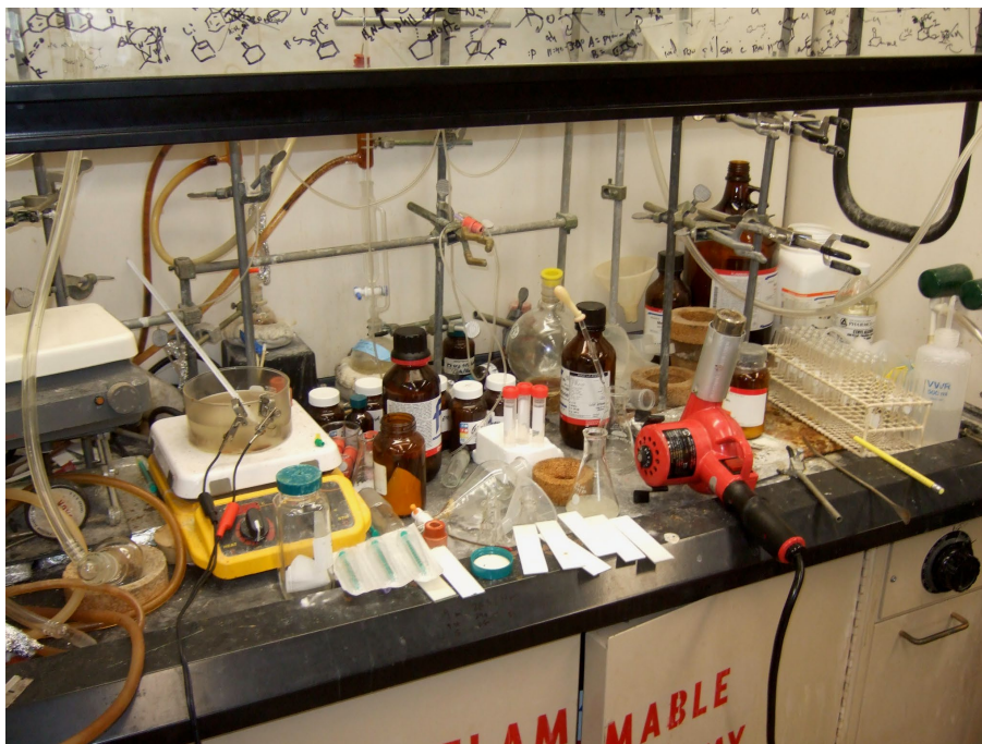
Figure 2 Poorly managed fume hood. Note the clutter and lack of elevation above the fume hood surface preventing adequate airflow. Additionally, the sash has been left up.
