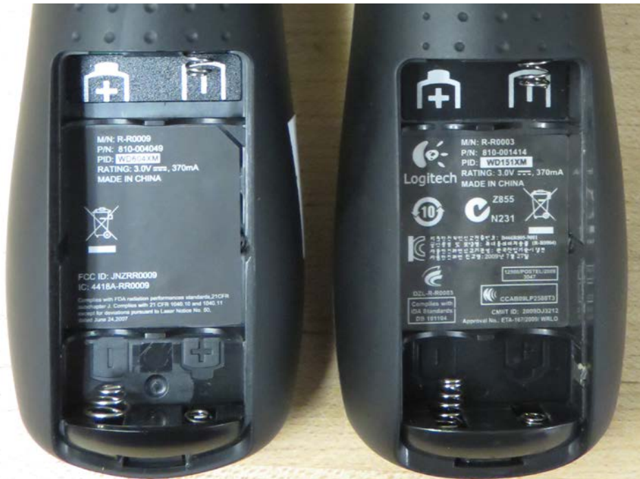
Figure 5: Internal Labels are Different (Counterfeit Pointer on Right)
