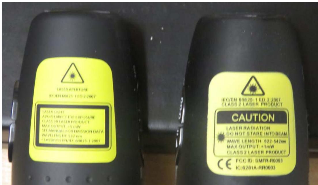
Figure 4: External Warning labels are Different (Counterfeit Pointer on Right)
