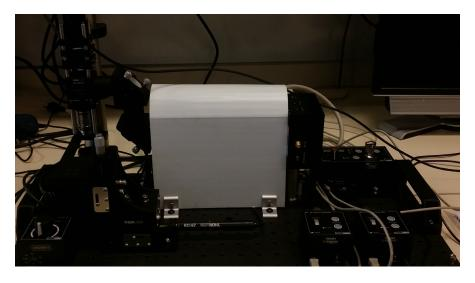
Figure 1: Coroplast® Cover Over Open Optical Path
